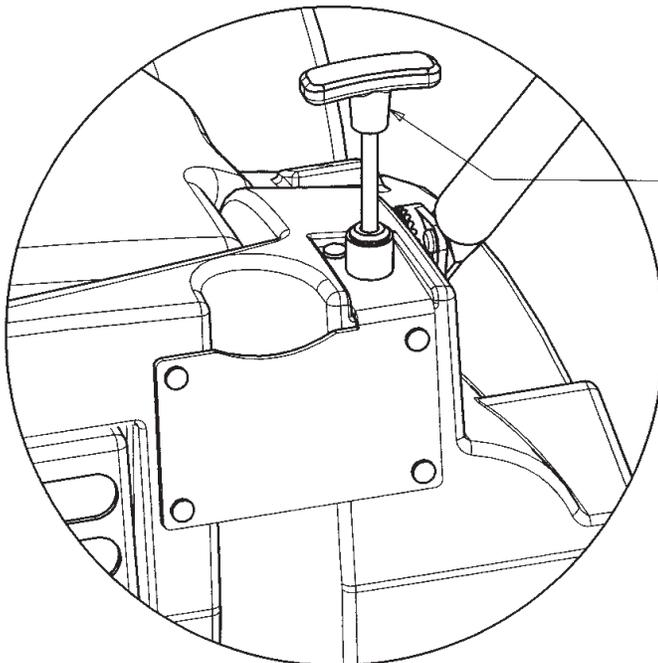
TURN AND LIFT HANDLE FOR OFF-AISLE WAND USE
