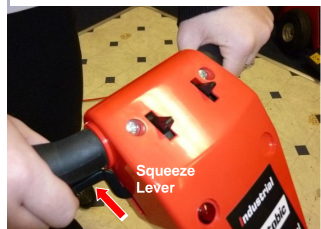
Pic 10 Squeeze Start / Run Lever to Operate
