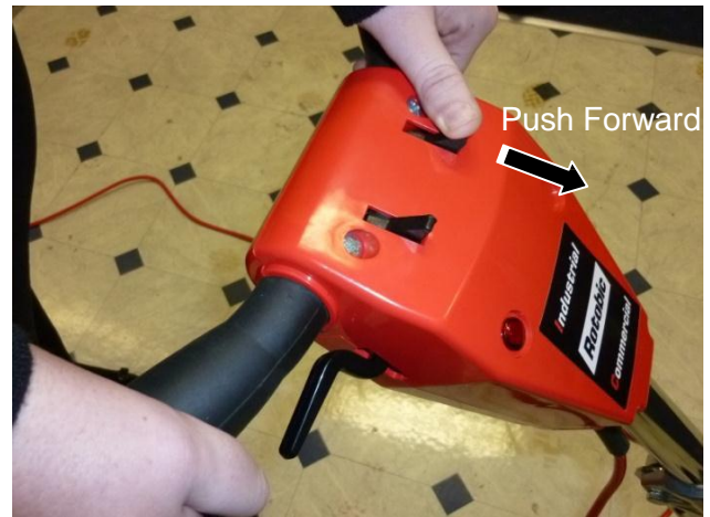
Pic 9 Dis-engaging the Safety Interlock
