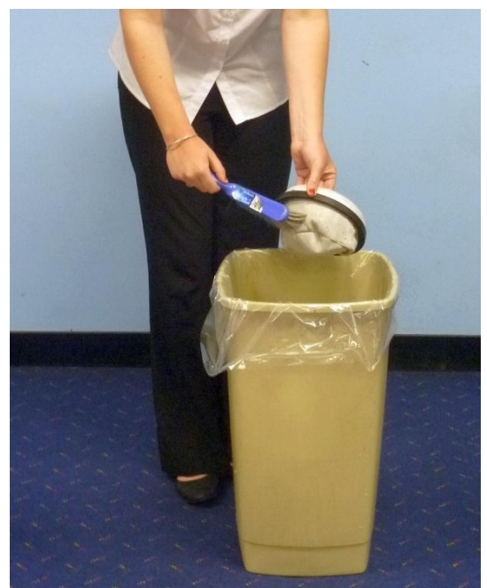
Pic 19 Filter Bag Maintenance
